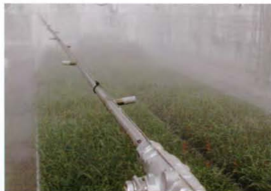
High-pressure stainless steel atomization lines deliver a fine mist which evaporates to provide cooling or humidification.
