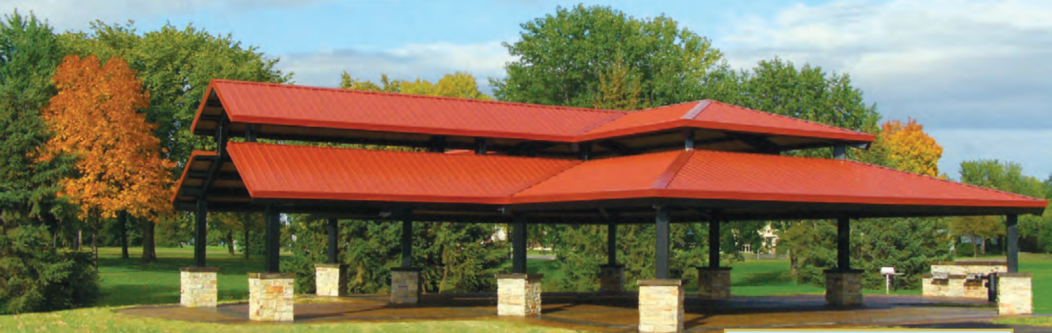
Model 8264DSM Custom 40'X64' Steel Beam Hipped Duo-Top "T" Shelter with 20'X40' Gable Extension, 4:12 roof pitch, 10" square steel columns and 29 gauge Litch-Top pre-cut metal roofing with 2"X6" Southern Yellow Pine T&G roof decking (masonry by others)
