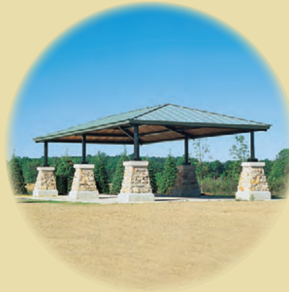
Model 8220SM-2 Custom 20'X44' Steel Frame Hip End with Western Red Cedar roof decking and standing seam metal roofing. Stone column pedestals designed and built by others.
