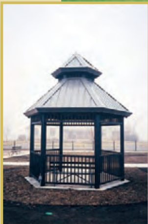
Model 7814SM 14' Steel Beam Kingsford Gazebo with overhead lattice, handrails, functional cupola and 2"X6" Southern Yellow Pine T&G roof decking over galvalume metal roofing
