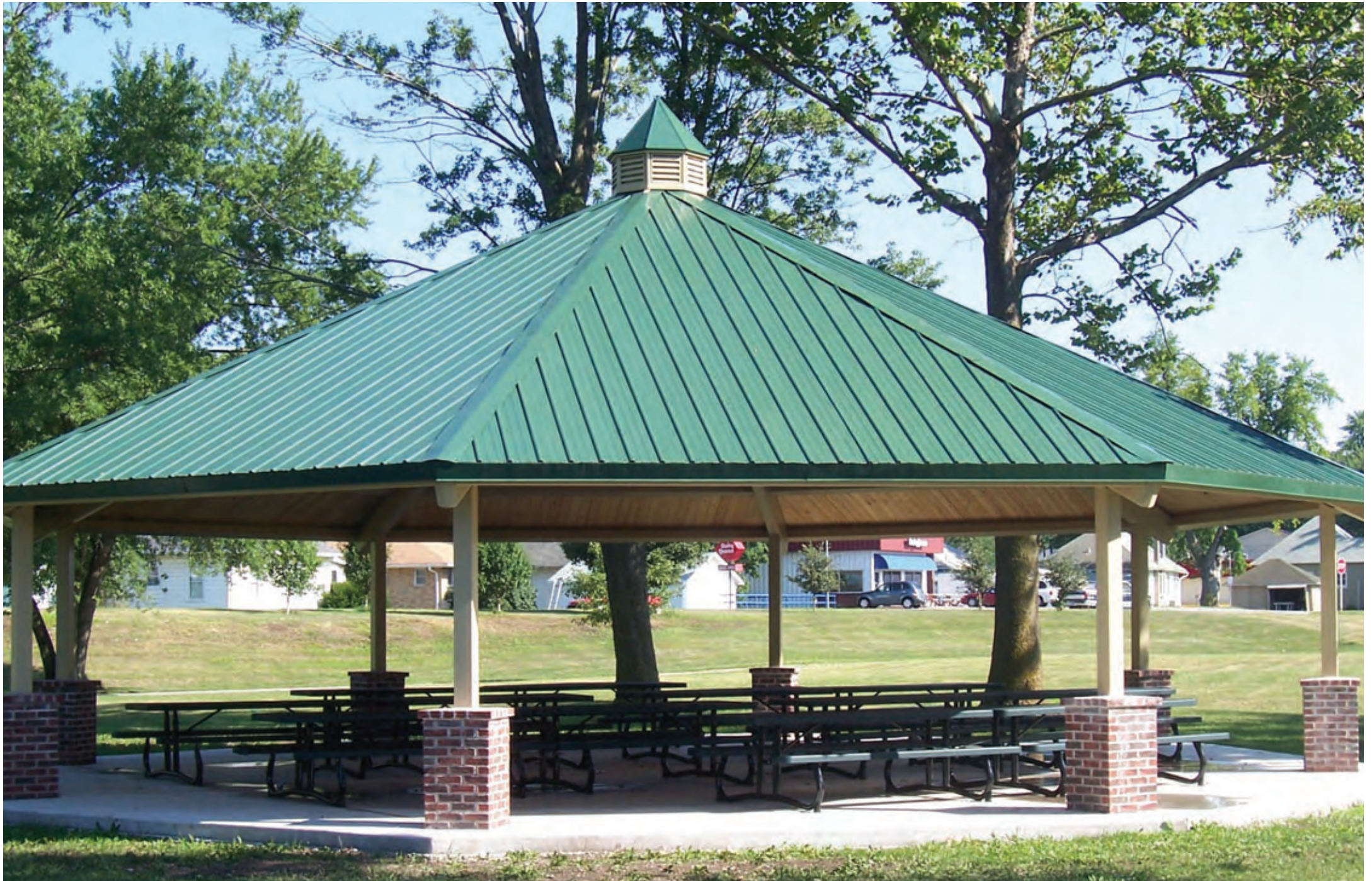
Model 8532SM Custom 32' Steel Frame Octagonal with cupola and 29 gauge Litch-Top pre-cut metal roof panels with 2"X6" Southern Yellow Pine roof decking. (column masonry by others)
