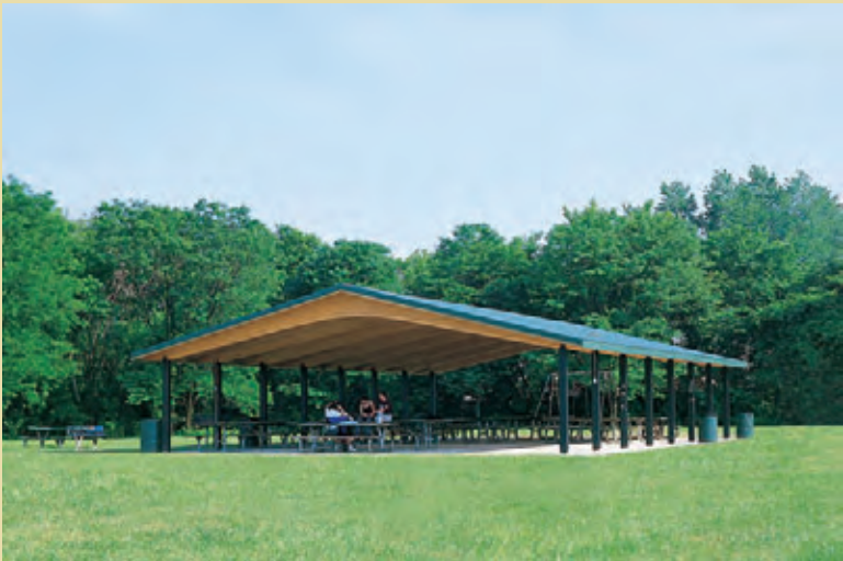
Model 1745 40' X 60' Laminated Curved Beam Gable End shelter with 2"X6" Southern Yellow Pine T&G roof decking, 29 gauge Litch-Top pre-cut metal roof and optional steel columns.
