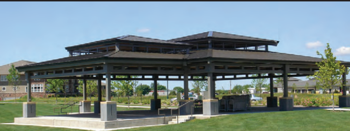
Model 8182P Custom Pittsburgh Performance Shelter utilizes a 50' Square Duo-Top adjoined to a 22'X36' Hip End Duo-Top which shares common supports with the 50' Square Duo-Top. Custom features include custom ornate laser-cut top tier lattice, custom column to beam connection and custom header lattice. Column masonry by others.
