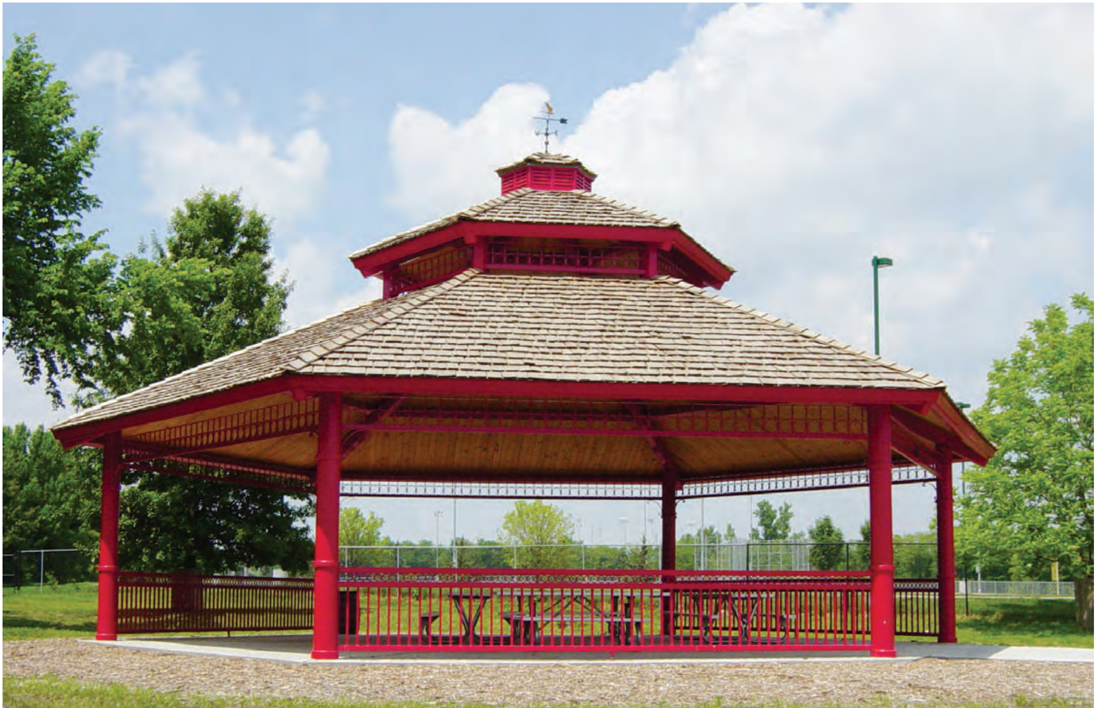
Model 8050S Custom 50' Steel Frame Hexagonal Duo-Top with custom laser-cut lattice & handrails, Cedar shakes (by others) over 2"X6" Southern Yellow Pine tongue & groove roof decking, round banded steel columns, cupola and weathervane
