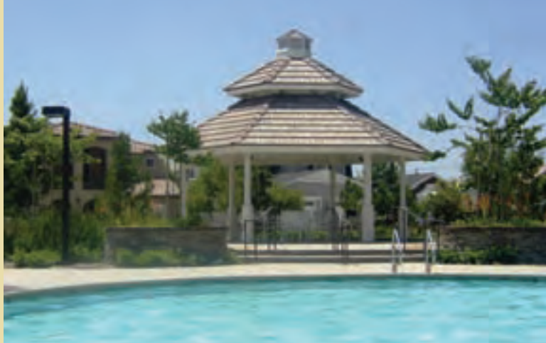
Model 7025 25' Deerfield Gazebo with glue laminated stepped columns, 2"x6" Southern Yellow Pine T&G roof decking and cupola (roofing material by others)
